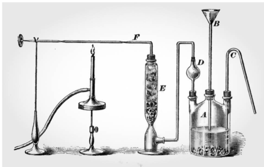
Figure 5. Apparatus for the Marsh test
