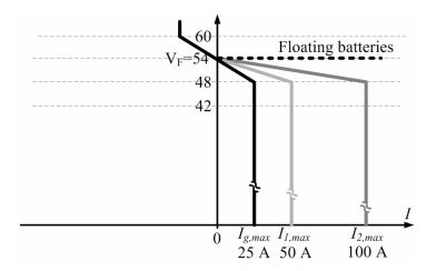
b) Now, the current increases to 120 A. What is the current output for each of the microturbines and for the grid interfacing converter (GIC)? What is the main bus voltage? What is the new no-load reference voltage for all droop lines? What is the batteries current? Draw the new droop graph.
