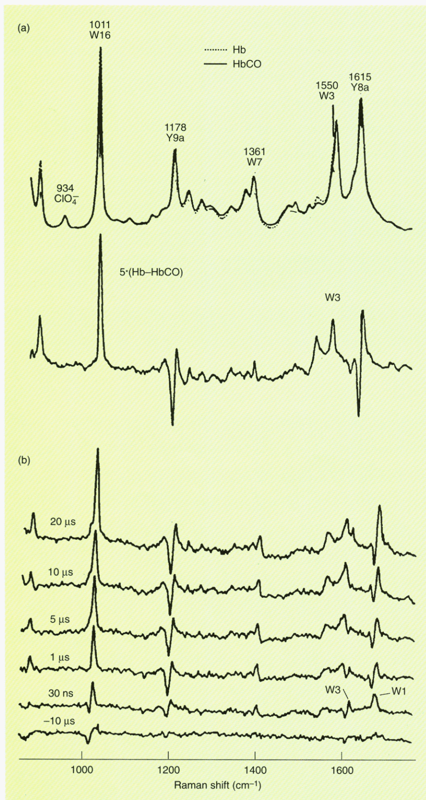
Figure 8. UV-Raman spectra of carbon monoxy- and deoxyhemoglobin excited at 230 nm.
