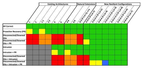
Fig. 2. Illustration of specific SCADA system configurations' ability to support the threat model we consider, including all combinations of a replica being unavailable due to proactive recovery, a site disconnection due to network attack or failure, and an intrusion (SCADA master compromise).
