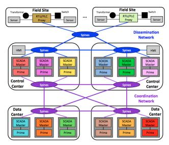
Fig. 6. Spire software architecture for configuration "3+3+3+3"
