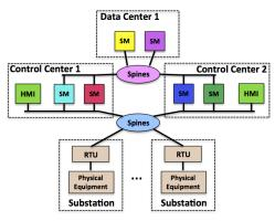
Fig. 4. SCADA Architecture with 2 replicas in each of the two control centers and the single data center (configuration 2+2+2).
