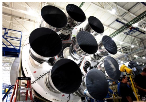
Figure 3 [15] Merlin Engines Used on a Falcon 9 Rocket
