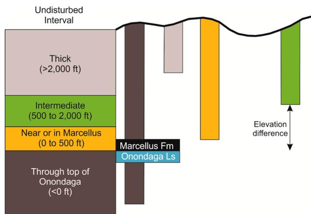
**Figure 3.** Simplified schematic illustrating the meaning of calculated undisturbed interval thickness between deepest vertical oil and gas well and top of the Onondaga Limestone. Interval bins and color scheme correspond to those in the histogram in Figure 5 and the raster pixel colors used in the map in Figure 4.
