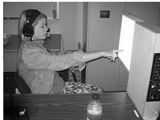
Fig. 1. Equipment setup with participant facing the stimuli presentations and the therein capacitance antennas housed behind the screen.
