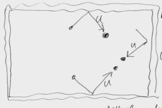
n molecules of mass m speed U, Uniformly distributed due all directions
