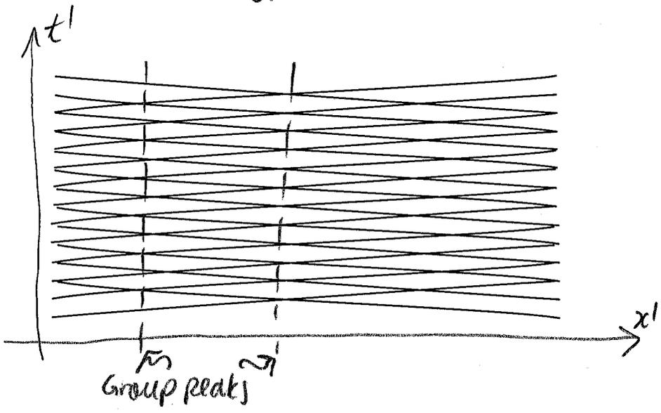
By symmetry, interference pattern produces a wave at rest.
