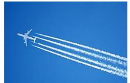
A high-flying jet's engines leaving a condensation trail (contrail)
