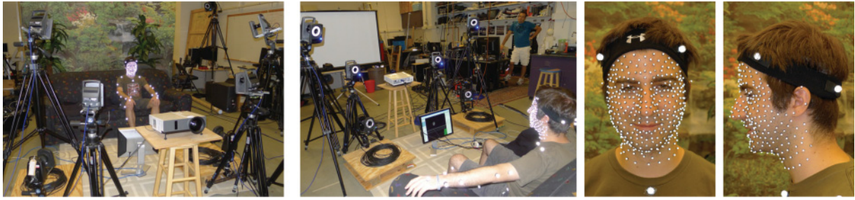
Fig. 3. Setup for recording smiles: facial motion was recorded with a commercial motion capture system that tracks the position of 250 3mm markers on the face.
