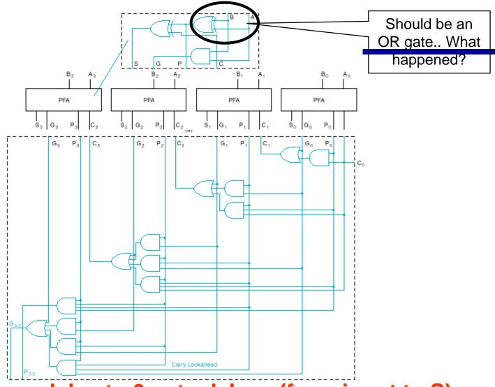
Reduces delay to 6 gate delays (from input to S)
