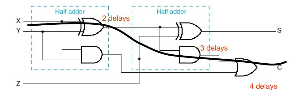
From Z to C is 2 delays for each subsequent stage or 2N + 2
