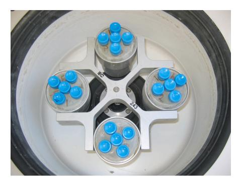
5) Set the centrifuge to the desired rotations per minute (RPM) and length of time to be centrifuged. For carbonate sample 1 minute at 4000 RPMs is generally adequate. **Do not adjust the rotor/radius**.
