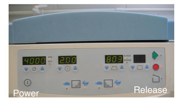
4) Place the inserts into the centrifuge cups. MAKE SURE THAT THE CENTRIFUE IS EQUALLY WEIGHTED ON ALL SIDES. If the centrifuge is not balanced, it will shut itself down.
