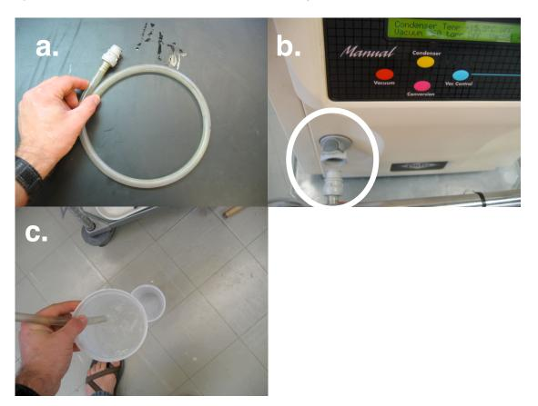
After using the freeze drier, you may speed up the melting process of ice in the condenser basin by pouring in a bucket or two worth of hot tap water. **DO NOT USE THE HEAT GUN TO MELT ICE IN THE CONDENSER**
