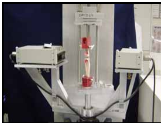
Figure 1. Laser micrometer with FMTC specimen while measuring CSA.
