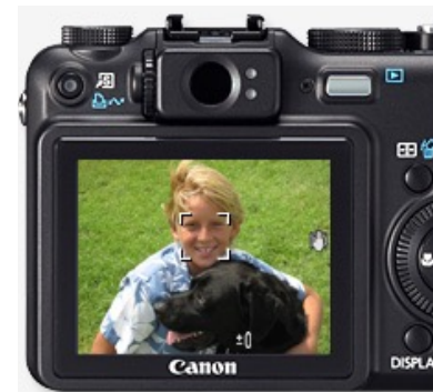
Setting camera focus via face detection
