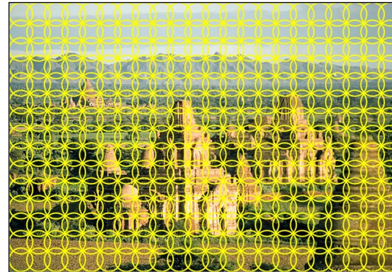
SIFT descriptors of 16x16 patches sampled on a regular grid, quantized to form visual vocabulary (size 200, 400)
