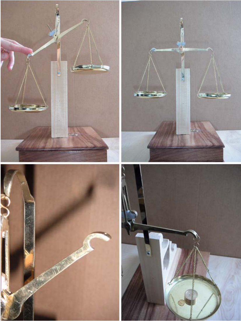
Fig. 21 The Jordanus balance. A considerable force is needed to keep the balance out of the horizontal position ( above left ). The balance in horizontal position ( above right ). Details of the mechanical setup of the connection ( below )
