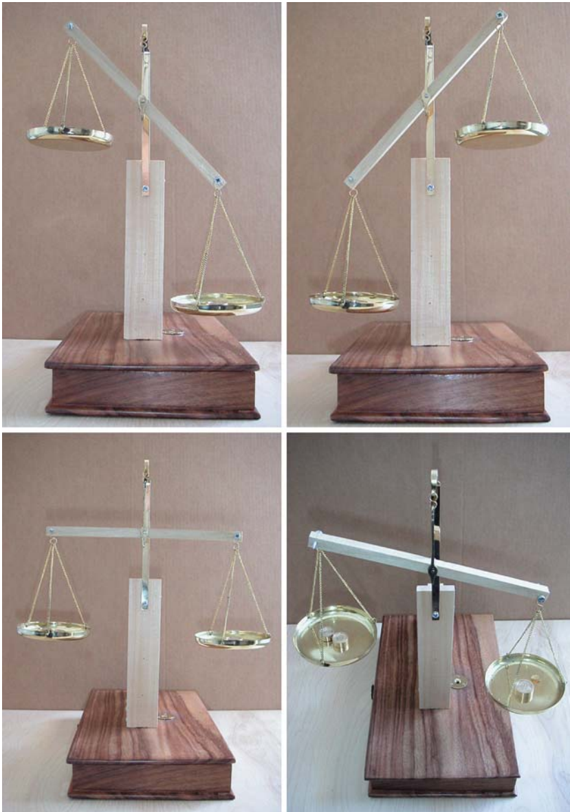
Fig. 22 The Guido Ubaldo balance. The balance in equilibrium in inclined positions (above left , and right ). The balance in equilibrium in the horizontal position (below left ), and in another inclined position from another angle (below, right ), showing coin-like weights
