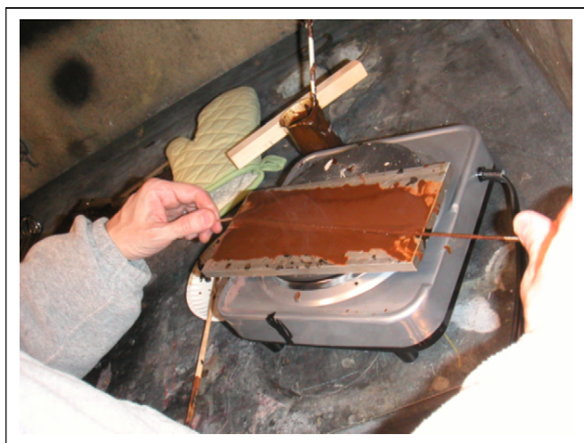
Figure 3. Learning how to make thin needles out of melted wax and a silk thread. We used a modern electric cooker to heat the wax, but at the beginning we tended to burn the delicate shellac all too easily before we finally figured that a constant, adequate temperature is best. What would Coulomb have used to keep his wax melted while trying to pass the silk thread into it to craft a needle? How do you let the wax set so that the needle will come out straight and not wavy?
