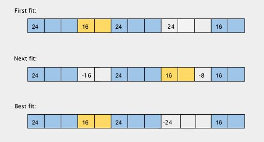
**First fit**: starts at beginning of heap and selects the first block that can be used
