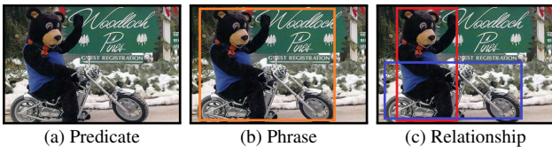
Figure 5: Detection Task Conditions: Given object bounding boxes: (a) Predicate (easy): does not require bounding boxes. (b) Phrase (moderate): requires relationship bounding box (orange) containing both objects. (c) Relationship (hard): requires individual bounding boxes (red/blue).
