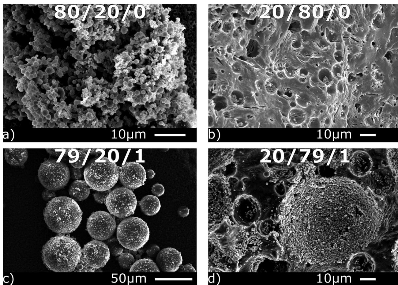
Fig. 2 SEM images of the effect of adding 1% DCDMS-coated particles on blends with PIB as the continuous phase (a and c) and PEO as continuous phase (b and d). The PIB/PEO/particle volume ratios are noted in each image.
