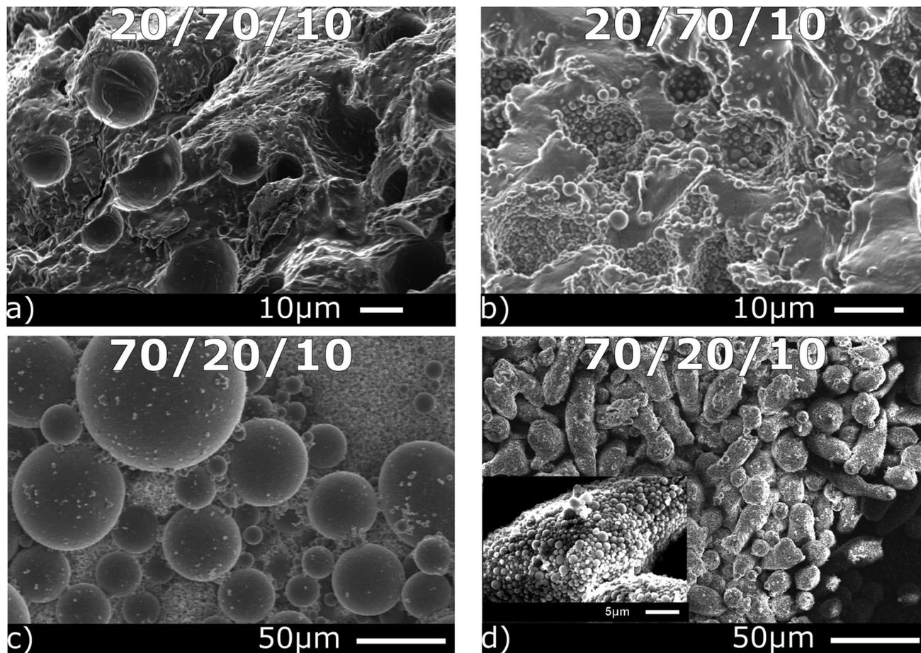
Fig. 1 SEM images comparing blends with unmodified silica particles (a and c) vs. blends with DCDMS-modified silica particles (b and d). The inset of (d) shows a higher magnification for the same blend to show the particles crowded at the interface. The numbers at the top of each image are the blend composition in the format of PIB/PEO/particle volume ratio.
