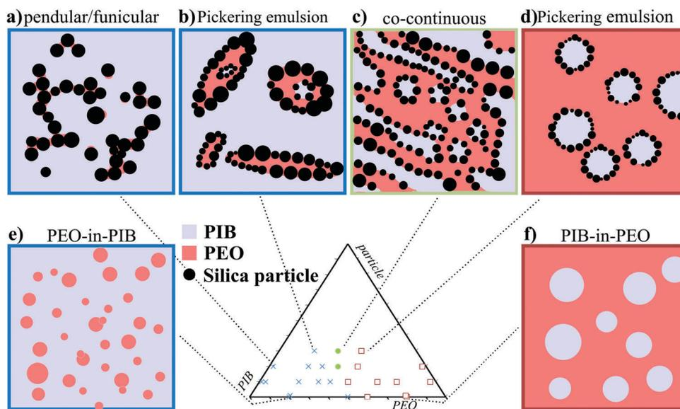
Fig. 6 A summary of all the composition studied and different morphology sketches at various compositions. From left to right: (a) pendular/funicular state when PEO is the minority phase; (b) PEO-in-PIB Pickering emulsion; (c) co-continuous state; (d) PIB-in-PEO Pickering emulsion; (e) PEO-in-PIB suspension; (f) PIB-in-PEO suspension.
