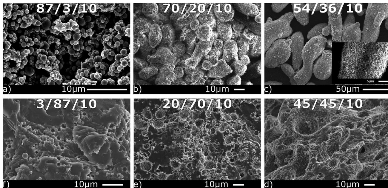
Fig. 3 Ternary blend morphology at various PIB/PEO/particle ratios listed in each image. The particle loading is 10% in all cases.
