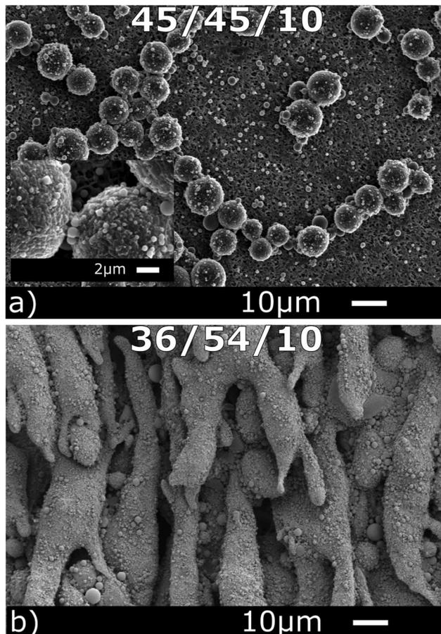
Fig. 5 Testing phase continuity of polymer blends containing OTS-modified silica particle at the two compositions (in the format PIB/PEO/silica) indicated in each image.
