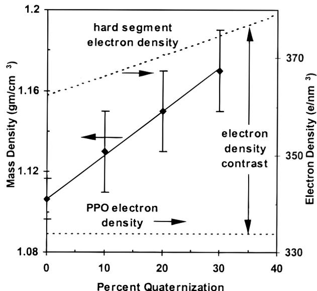
**Figure 5.** Effect of the extent of quaternization on the mass and electron density of the hard segments of polyurethane cationomers. Solid diamonds and solid line refer to the left axis whereas the broken lines refer to the right-hand axis.
