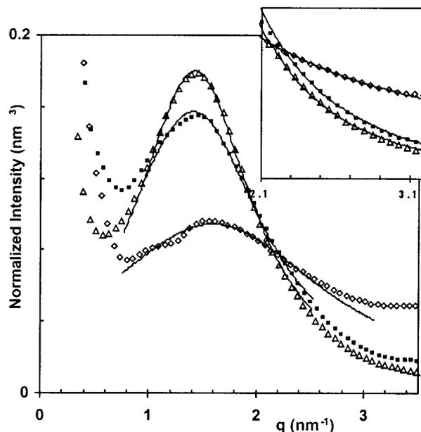
**Figure 6.** SAXS data for the I725 series collected at room temperature:  $\diamond$ , I725-12;  $\blacksquare$ , I725-25;  $\triangle$ , I725-40. Data have been normalized by the square of the electron density contrast. Only 20% of the data points have been shown. Solid lines are Lorentzian fits to the peaks. The inset shows a magnified view of the data at high  $q$  and the power law fits to eq 10.
