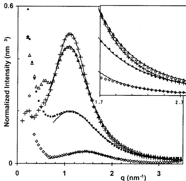
**Figure 7.** SAXS data for the I1000 series collected at room temperature:  $\diamond$ , I1000-0;  $\blacksquare$ , I1000-13;  $\triangle$ , I1000-32;  $+$ , I1000-40. Data have been normalized by the square of the electron density contrast. Only 20% of the data points have been shown. Solid lines are Lorentzian fits to the peaks. The inset shows a magnified view of the data at high  $q$  and the power law fits to eq 10.
