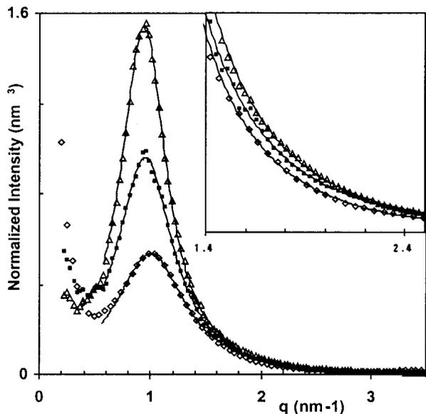
**Figure 8.** SAXS data for the I2000 series collected at room temperature:  $\diamond$ , I2000-0;  $\blacksquare$ , I2000-14;  $\triangle$ , I2000-20. Data have been normalized by the square of the electron density contrast. Only 20% of the data points have been shown. Solid lines are Lorentzian fits to the peaks. The inset shows a magnified view of the data at high  $q$  and the power law fits to eq 10.
