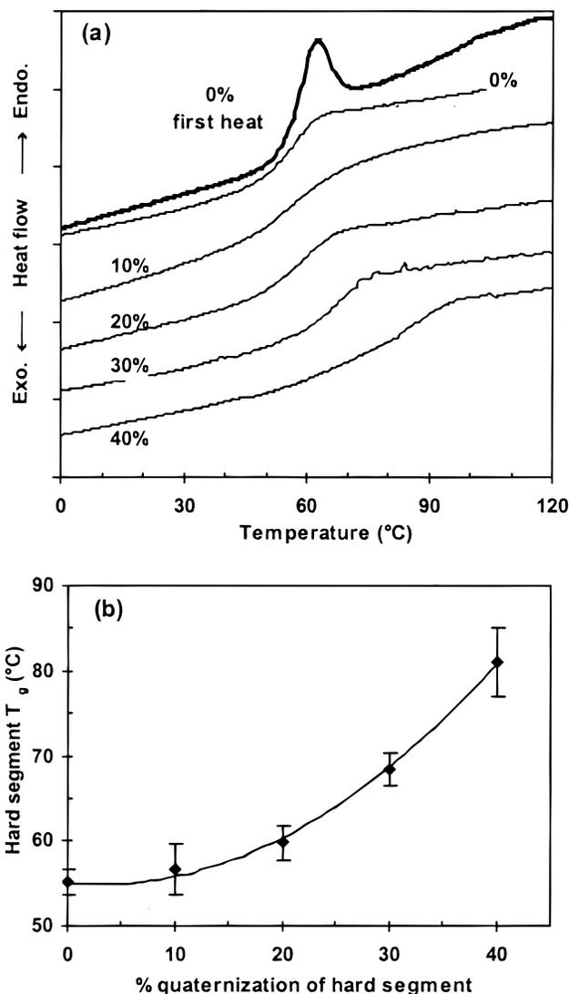
**Figure 1.** Effect of the extent of quaternization on the hard-segment  $T_g$ . (a) DSC traces of pure hard segments with various degrees of quaternization: top curve is first heat; all others are cooled from 140 °C. Each tic on the  $y$ -axis is 0.2 J/(g K). (b)  $T_g$ 's measured from second heat traces in (a) and a quadratic fit.
