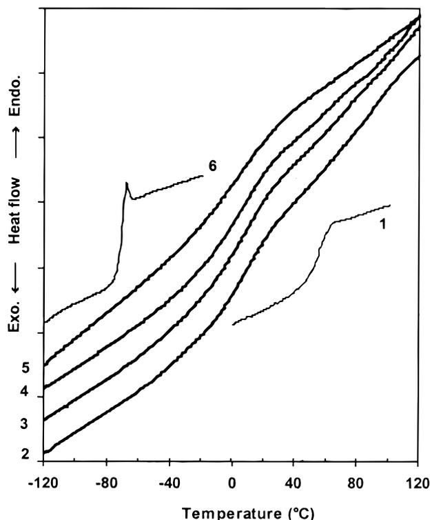
**Figure 2.** DSC traces of I725 series. Curves correspond to (1) pure IPDI/DMP, (2) I725-0, (3) I725-12, (4) I725-25, (5) I725-40, and (6) pure soft-segment PPO-830. Each tic on the y-axis is 0.2 J/(g K). All data shown are first heats. Annealing at 55 or 140 °C produces identical traces. Note that trace 1 refers to the hard segment of the unquaternized PU only. All other PUs have higher hard-segment  $T_g$ 's as per Figure 1.
