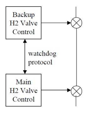
If the handshake fails, then either one or both can shut off the gas supply. Is this a single fault tolerant system?
