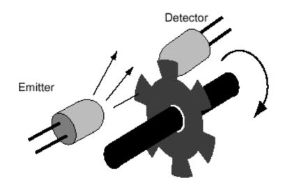
Tachometer: RPM measurement
