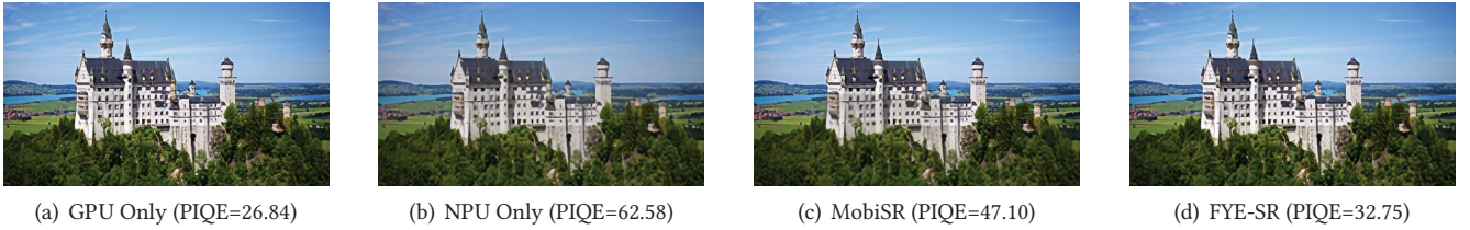
Figure 16: Samples of upscaled images using ESRGAN model with 4\times 720\times 480 output. FYE-SR can effectively suppress the distortions and visual inconsistency at detailed objects (windows on buildings).
